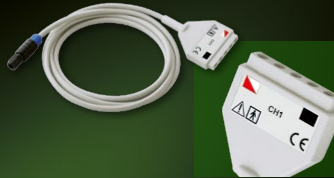
41-0073 Stimulation cable for TWISTER® MM and AVALANCHE® PLUS I/O box 1-channel, output 1-4, for connection of stimulation probes and electrodes, with DIN 42802-1 connectors, cable length 4 m, connector blue/black, not autoclavable
