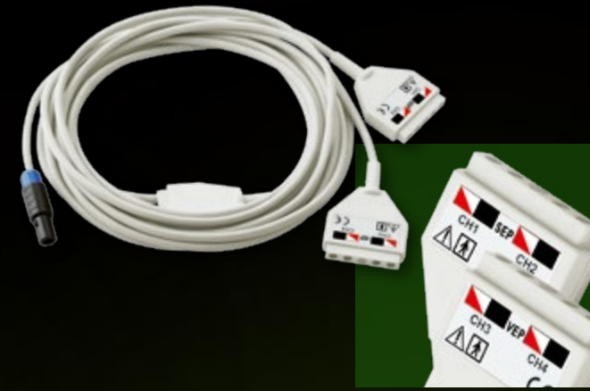
41-1000 Stimulation cable for AVALANCHE® PLUS I/O box for connection of stimulation probes and electrodes with DIN 42802-1 connectors (output A1-2) and VEP flash goggles with DIN 42802-1 connectors (output A3-4), cable length 4 m, connector blue/black, not autoclavable
