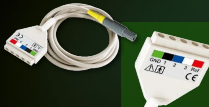
41-0020 EP recording cable 3-channel, active, for AVALANCHE® headbox, for connection of electrodes with DIN 42802-1 connectors, cable length 1.5 m, shielded, connector yellow/grey, not autoclavable
